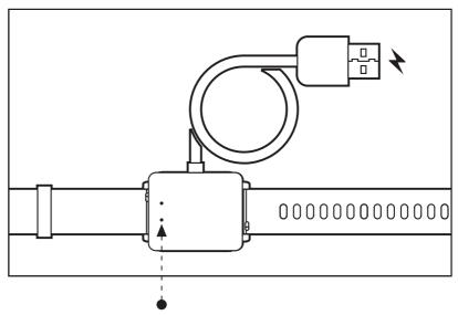
When charging, ensure that the charging contact points on the fitness tracker and the magnetic cradle are aligned.
